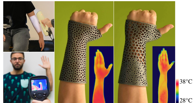
Figure 1. We propose a new method for thermal-comfort design of personalized casts. (Left) Physical-data acquisition by a 3D scanner and a thermal camera. (Right) Comparison of skin temperature on uniform skin exposure (left) vs. our optimized cast (right). Two casts have the same area of skin exposure.
