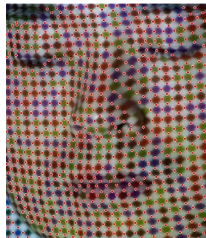
Figure 6. Grid-point detection result on a real human face with pattern illumination.
