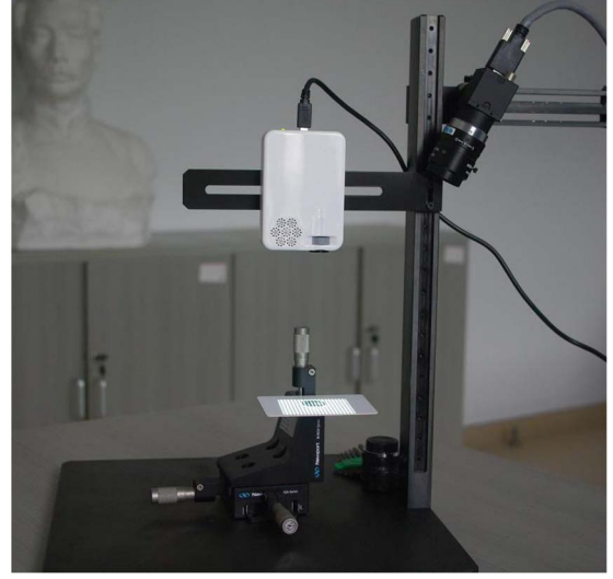
Fig. 6. Experimental setup consists of an off-the-shelf pico-projector and a camera, and the two devices are synchronized.
